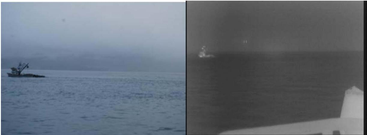
Note in Figure 2, we see not only the obvious fishing vessel in 10-14 micron LWIR, but also the engines and exhaust system of the Supertanker at the TAP (Trans Alaska Pipeline), which is more evident with a narrower field of view as shown in Figure 3, but still obscured by fog. With image fusion, the thermally hot pixels in the LWIR image can be overlaid on the visible image in a single image with proper image registration and resolution matching.
