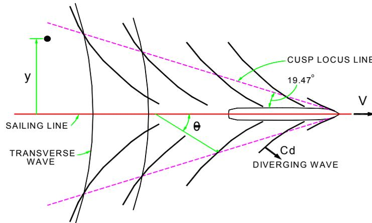
Figure 1. Definition sketch showing plan-form of ship-generated waves
