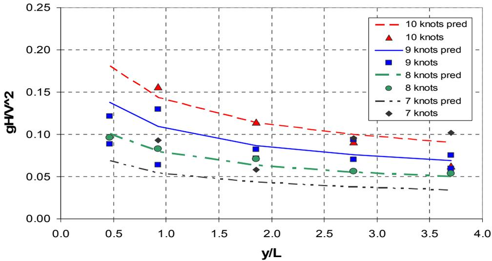
Figure 6 Results of the field trials along with prediction using new empirical model in equations (1) through (4).
