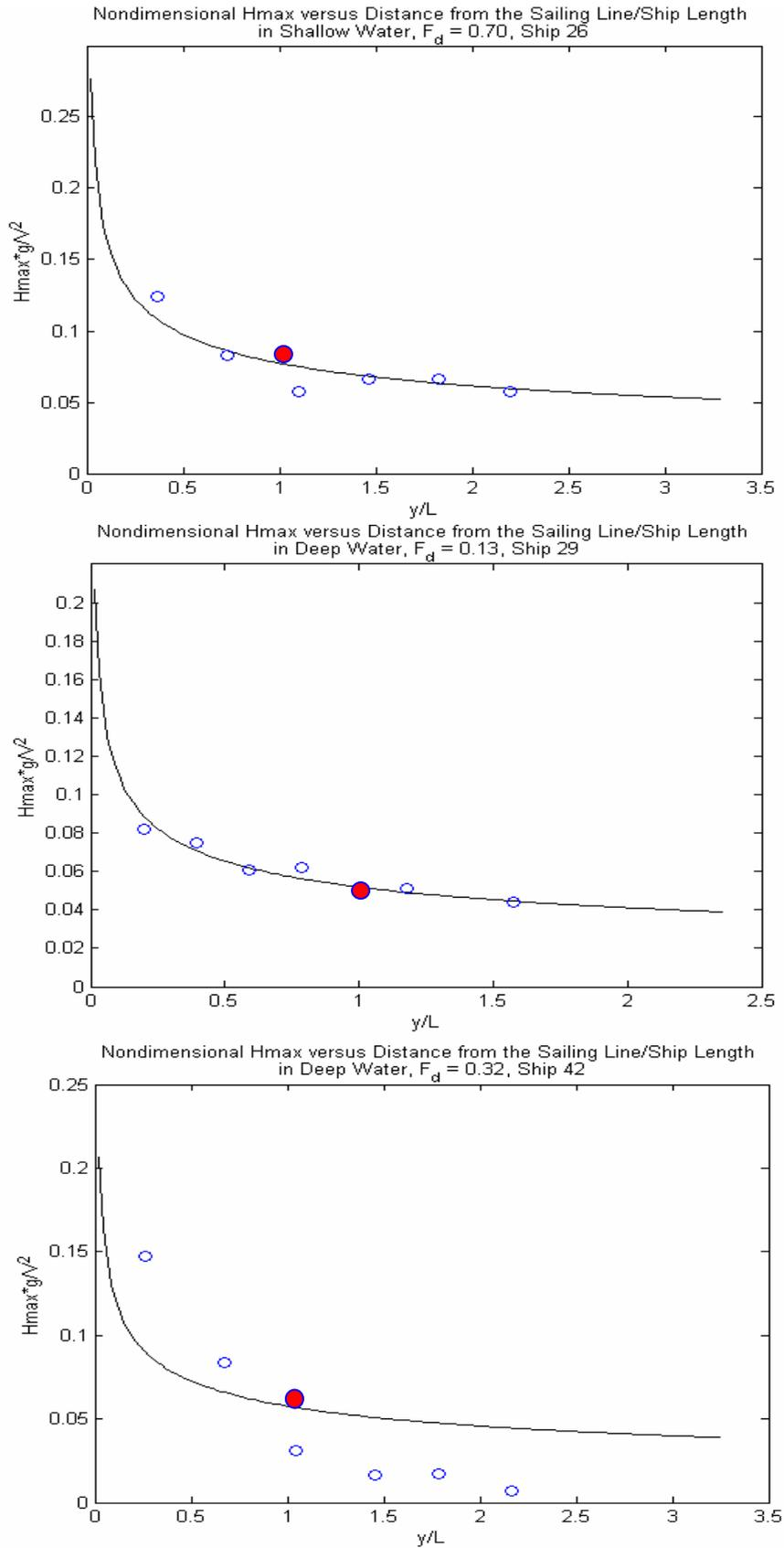
Figure 2. Examples of wave height decay with distance from sailing line.
