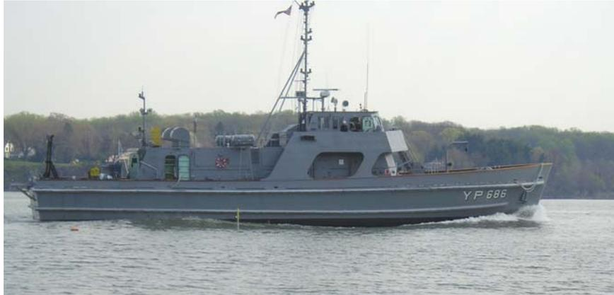
Figure 5. Vessel used in field trials, the YP686. Vessel is shown passing wave gage. The wave staff is visible just aft of midships.
