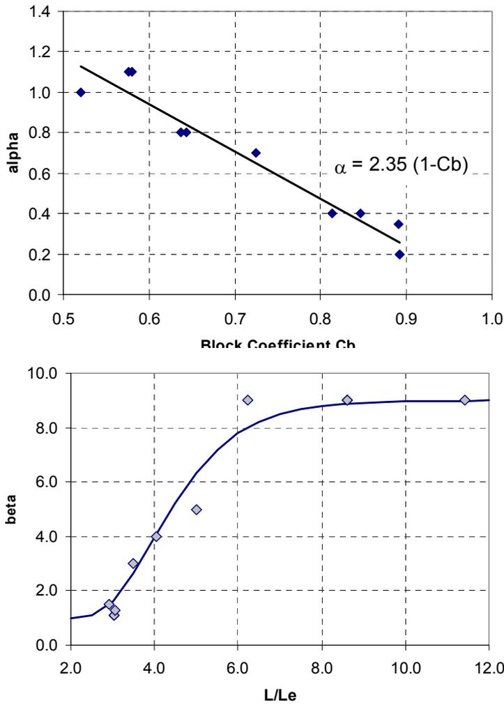
Figure 4. Top figure (a) showing parameter  $\alpha$  used to define the modified Froude number. Bottom figure (b) showing the parameter  $\beta$  used to define the rate of increase of  $gH/V^2$  with the modified Froude number.
