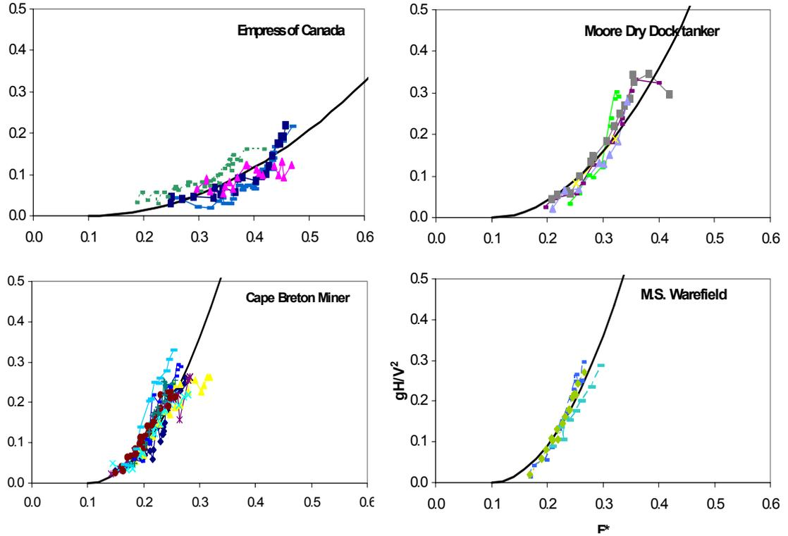
Figure 3. Examples of  $gH/V^2$  at  $y/L=1$  plotted versus modified Froude number  $F^*$ . For each ship, the use of  $F^*$  seems to collapse results from many depth-to-draft ratios (different symbols/colors) to a single curve. Also shown are best-fit quadratic curves for  $F^*>0.1$ .
