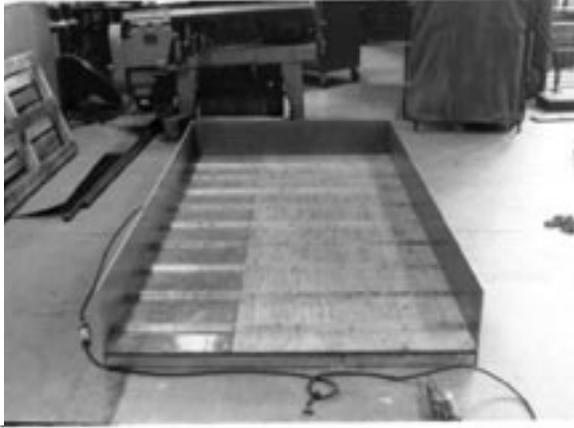
Figure 6. Aluminum box used for model riprap bank.
