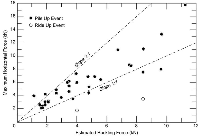
Figure 23. Plot of maximum force recorded during each test vs.  $b\rho_w g L^2$ , where  $b$  is the width of ice sheet,  $\rho_w g$  is the specific weight of water, and  $L$  is the characteristic length of floating ice sheet.
