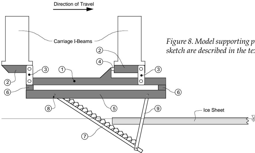
Figure 8. Model supporting platform. Items numbered in this sketch are described in the text.
